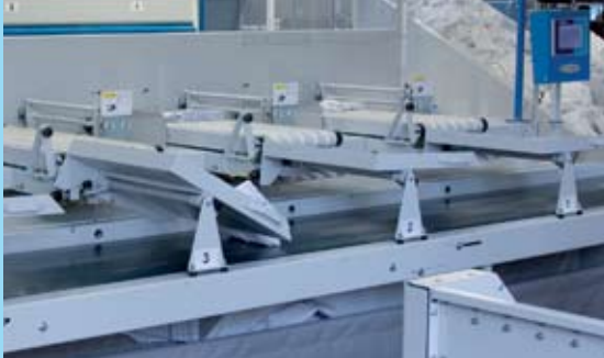
Tilt tray system with conveyor (option)
